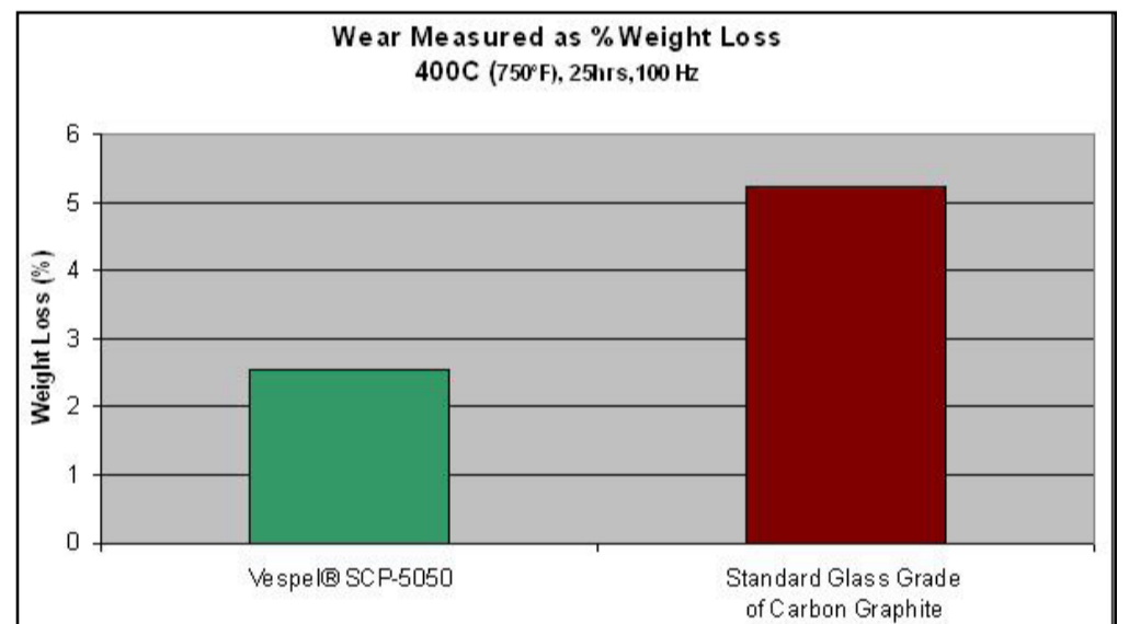
Figure 2: Test Method: Oscillating wear comparison with 2.27 kg (5 lb) load at 100 Hz for 24 hr
